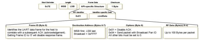
Note: the Frame ID byte has no impact on the communications between the PAC and the LOBBYIST. It is only used to identify which outgoing packet an XBee status message refers to. It's required that the LOBBYIST receives a confirmation of receipt from the PAC's XBee before rotating the its encryption key. For that, the Frame ID has to be used but this document does not impose any implementation details.
